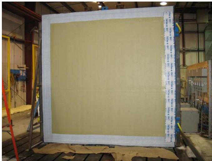
Figure D-2 – Completed Air Barrier Installation (Sheathing Joints Sealed, Second Coat of LATICRETE Air & Water Barrier Applied and LATICRETE Transition Tape and LATICRETE Flexible Sealing Tape Applied)
