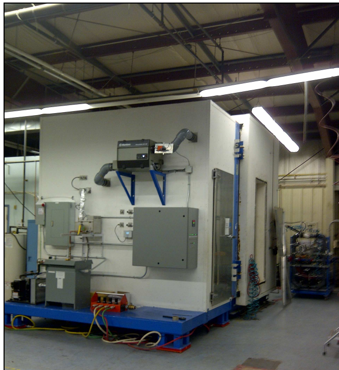
Figure 2 – General Specimen Installation between Warm Side and Hygrothermal Chamber
